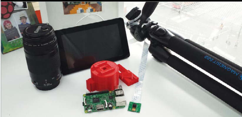
Above All the components James used for the project, including the red 3D printed lens adapter in three parts, which he later wrapped in duct tape
