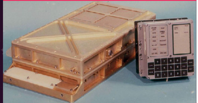
The AGC computer and its control pad. Computers were very different in the Sixties, relying mostly on magnetic ribbon for storage
